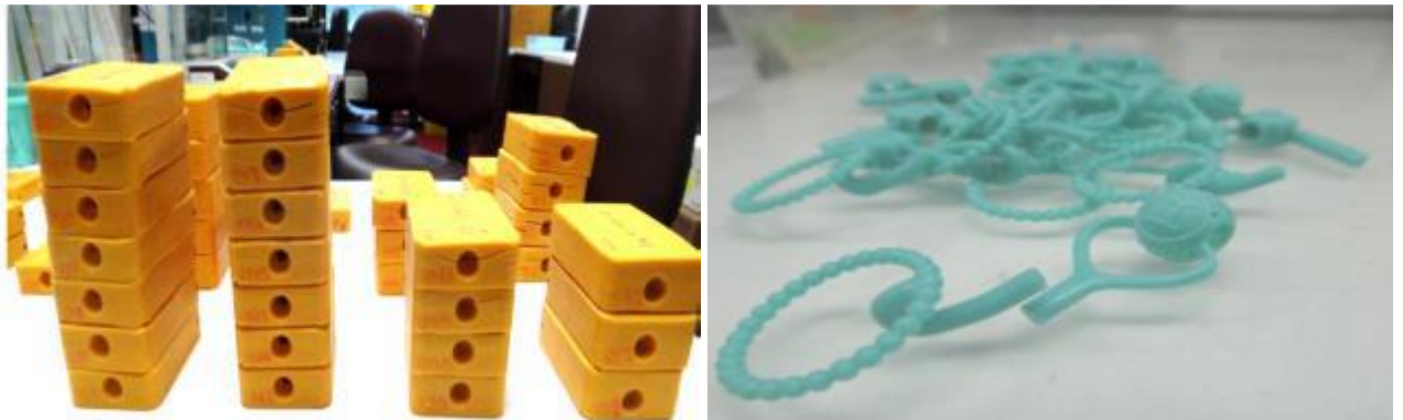
Figure 4 Reusable rubber moulds and wax copies of charms and other jewels including the holder.
